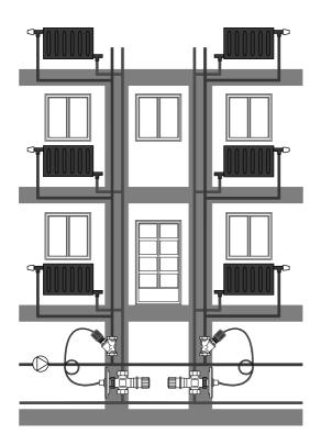
Fig. 2. Stop Valve-3 as supply shutoff valve and impulse tube connection with a Kombi-PC in a two-pipe system
