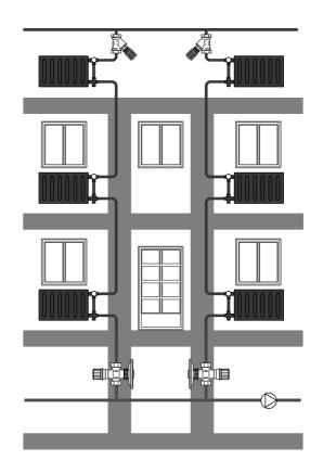
Fig. 3. Stop Valve-3 as supply shutoff valve with a Kombi-FC in a vertical one-pipe system
