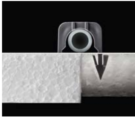
Minimal pipe lifting due to x-net pipe anchors.
